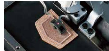
The device is best-suited to attaching small articles such as labels and emblems by sewing the entire circumference.
