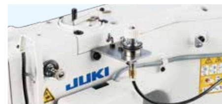
The tension controller unit used to partially change the needle thread tension during the sewig of a pattern.
