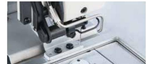
The needle cooler blows air to the needle, thereby preventing thread breakage caused by hot needles.
